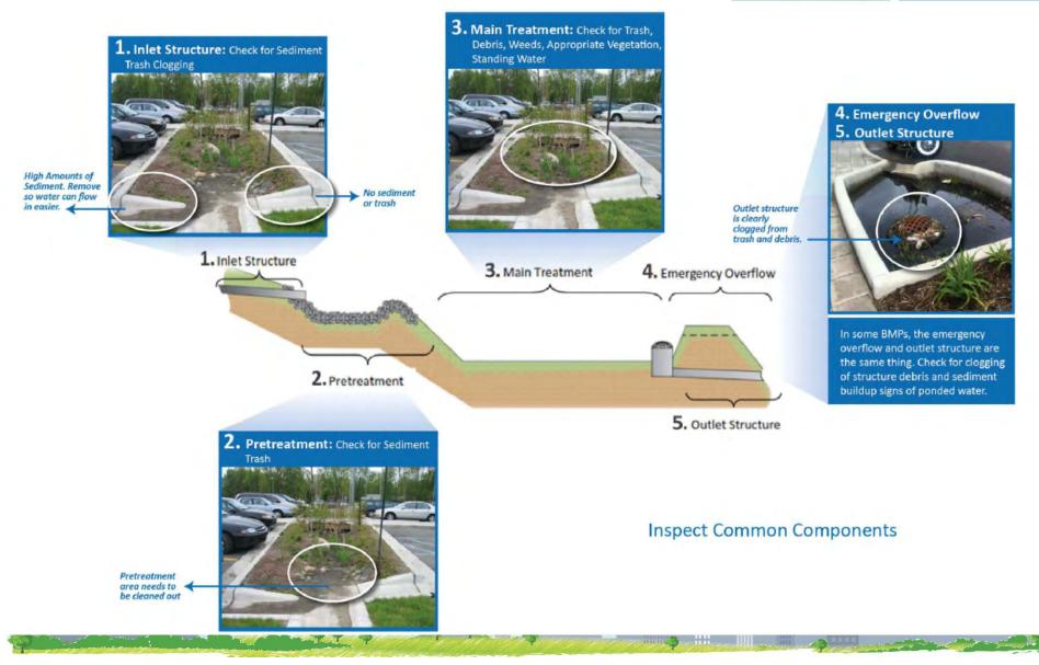
Inlet structures bring water into the BMP. They should be free of sediment, trash, and debris. Erosion, scour, and damage should be evaluated.
